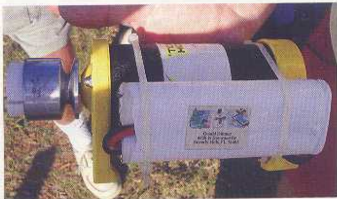
Above: The A123 four-cell pack makes a great starter battery.
