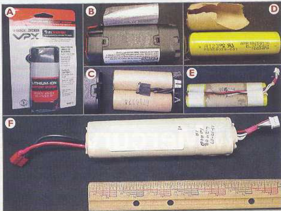
Building a four-cell pack from A123 cells. C: Cells removed from shell. D: Paper sleeve is saved for pack assembly. E: Pair of cells folded to form two sticks and paper sleeve over each stick. F: Completed pack with heat shrink.
