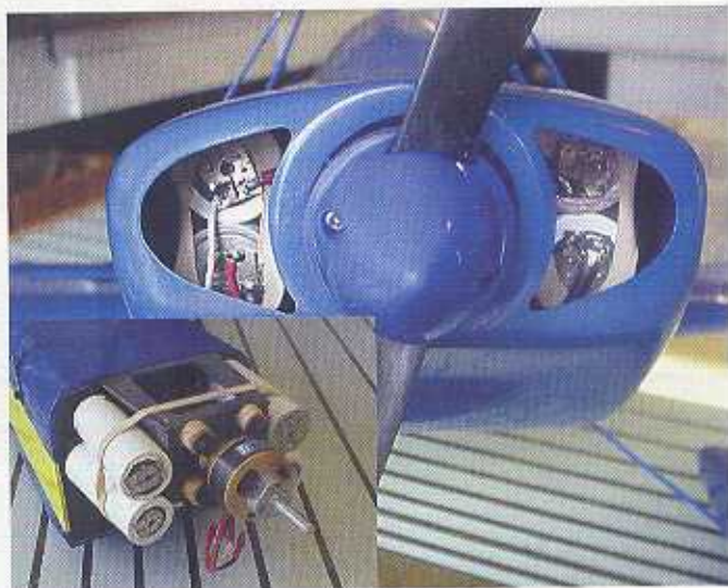
Right: A 4S A123 pack in the author's Ultimate biplane brings the CG into the proper location.
