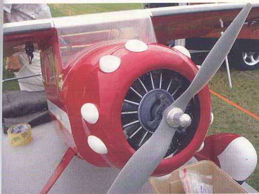
This Giant Scale Monocoupe was converted to electric power.
